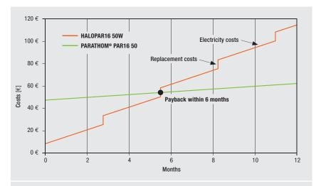
Fig. 4. The replacement of halogen reflector lamps by PARATHOM PRO PAR16 50 LED lamps pays off after just six months. The calculation is based on an electricity price of  $\leqslant$ 0.17/kWh, an operating time of 24 h/d, and replacement costs of  $\leqslant$ 8 each for lamp and manpower
