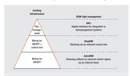
Fig. 2. OT 65 3DIM and PTo 3DIM control gear offers various dimming capabilities in combination with existing infrastructure
