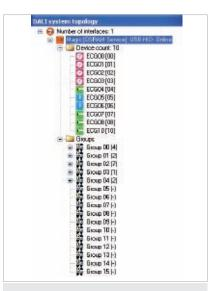
Fig. 4. Visualisation of the DALI lighting installation as a tree structure
